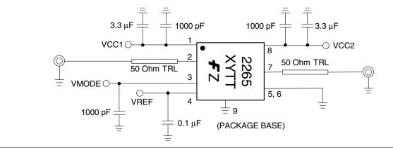
RMPA2265 Dual Band WCDMA Power Edge™ Power Amplifier Module 1850 to 1910 MHz and 1920 to 1980 MHz
